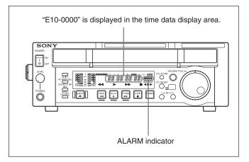
If this happens, the drum and capstan motors stop and the cassette is automatically ejected. Then, the drum starts to rotate again to dry its surface. In this state, the unit is not operable. When the moisture has evaporated, the ALARM indicator goes off and the "E10-0000" message disappears.
